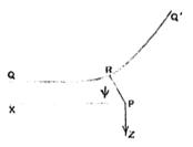
place, and since the encounters are assumed to be binary, m describes a symmetrical curved path QRQ', R being the apse. Let the angle  $XPR = \psi$ . The whole effect of the encounter, so far as regards the change of direction of the motion of m, is the same as if m received an impulse  $2mq\cos\psi$  in direction PR. Then also P experiences an impulse  $2mq\cos\psi$  in direction RP.
